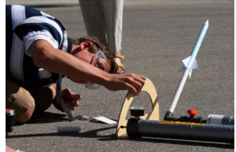
2. Attach the bike pump to the launcher, and pump to predetermined pressure (typically 50 psi).
