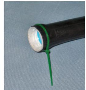
3. Attach the other end of the inner tube to the PVC pipe.
